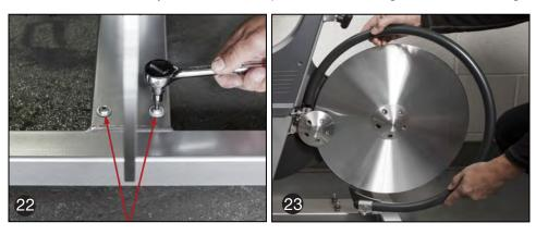
Step 5: Swing the tube over the flywheel, aligning the tube centered with the flywheel.
