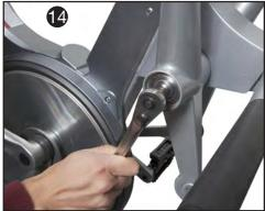
Step 3: Align and assemble the Handle to the link as shown (Fig. 15). While holding the 6mm Allen Wrench on the Socket Button Head Cap Screw (N6), Tighten and torque the Hex Elastic Lock Nut (N4) to 23 Nm (17 ft-lbs) using a 17mm socket and torque wrench.
