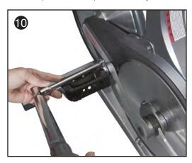
Step 2: With a clean cloth, wipe the threaded area of the pedals. Apply Loctite 242 to the pedal threads. Install the pedals into the crank arms, use the 15mm open-end wrench to tighten. Finish with the torque wrench, 15mm crowfoot, and 6" extension. Torque pedals to 47 Nm (35 ft-lbs) (Fig. 10).
